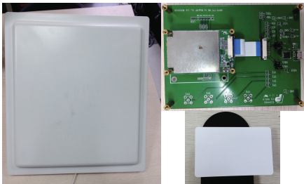
Fig. 1. RFID components, consists of a passive tag, a platelike antenna and a pan-tilt unit
